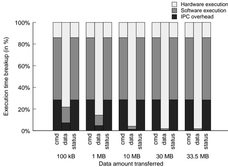
Figure 11.4: Break up of read command execution stages
