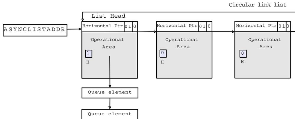
Figure 5.3: Asynchronous queue in host controller
