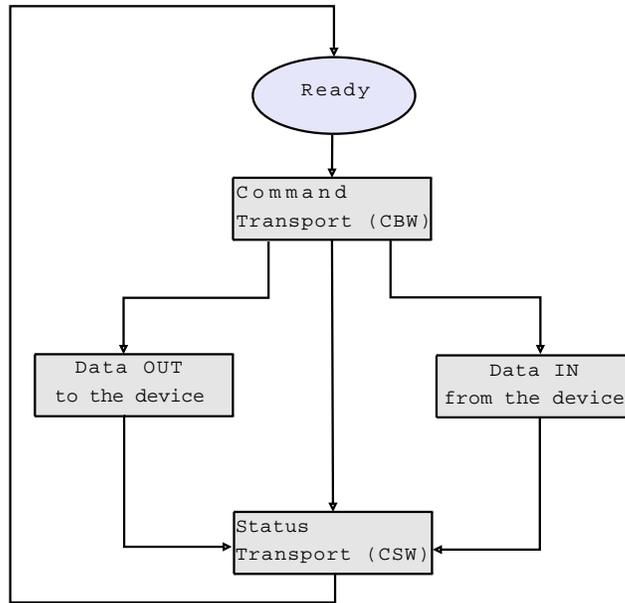
Figure 10.1: Command/Data/Status Flow
